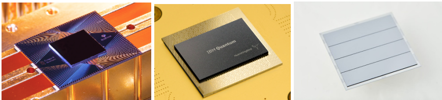
Figure 5.7: Superconducting processors (l to r): Google, IBM, Rigetti Source (l to r): Google, [164], [274]
